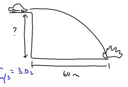
$$\frac{Vertical}{\vec{a}_{S} = 9.8 \text{ m/s}^{2} \text{ (down)}} \qquad \frac{\vec{\Delta}_{d} = \vec{V}_{1} \cdot D_{t} + \frac{1}{2} \vec{a}_{t} (\Delta t)^{2}}{\vec{\Delta}_{S} = 9.8 \text{ m/s}^{2} \text{ (down)}} \qquad = 0 + \frac{1}{2} (9.8)(3)^{2}$$
